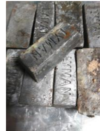
Old dirty lead ingots will need to be re-melted and cleaned before placing them in the Oasis Lead Shot Maker.
