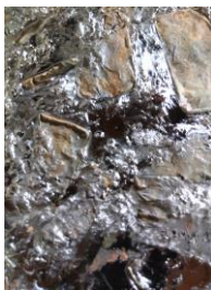
Notice how the crud and debris float to the top of the melted lead, clean this scum off before using.
